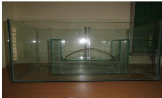
Fig. 2 : Sample under testing for hygric strain measurement.
